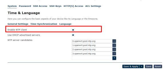
Notice: As using NTP server, as webpage time count will be slower than the device time, please refresh the webpage or use the SSH command to confirm the device time.
