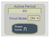
User can set up the time and the final status in power cycle as ON / OFF.
