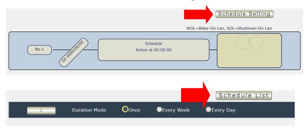
The schedule allows you to control the power outlet turn ON, OFF, Cycle, WOL, SOL or Reboot at the assigned time user arrange in schedule
