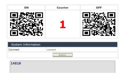
Scanning on and off QR code will trigger the IO control, and will show their command code below.
