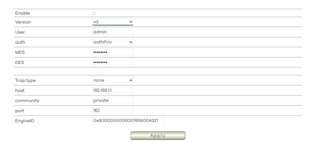
(1) auth: this function provide the certified and encryption to the device.
