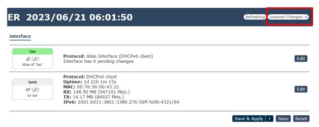
Click the Unsaved changes you will see the small screen shows "Configuration / Changes ". It show the section you have added, changed or removed, the changes based on different colors to show how many section you want apply.
