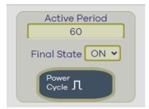
User can set up the time and the final status in power cycle as ON / OFF.
